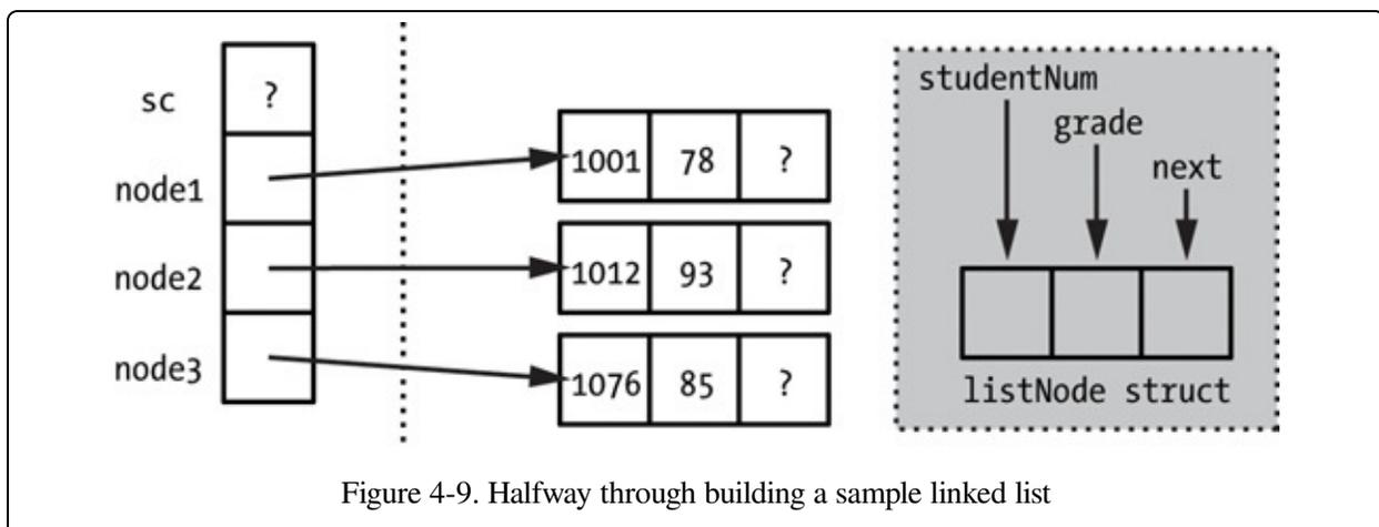
Figure 4-9. Halfway through building a sample linked list
