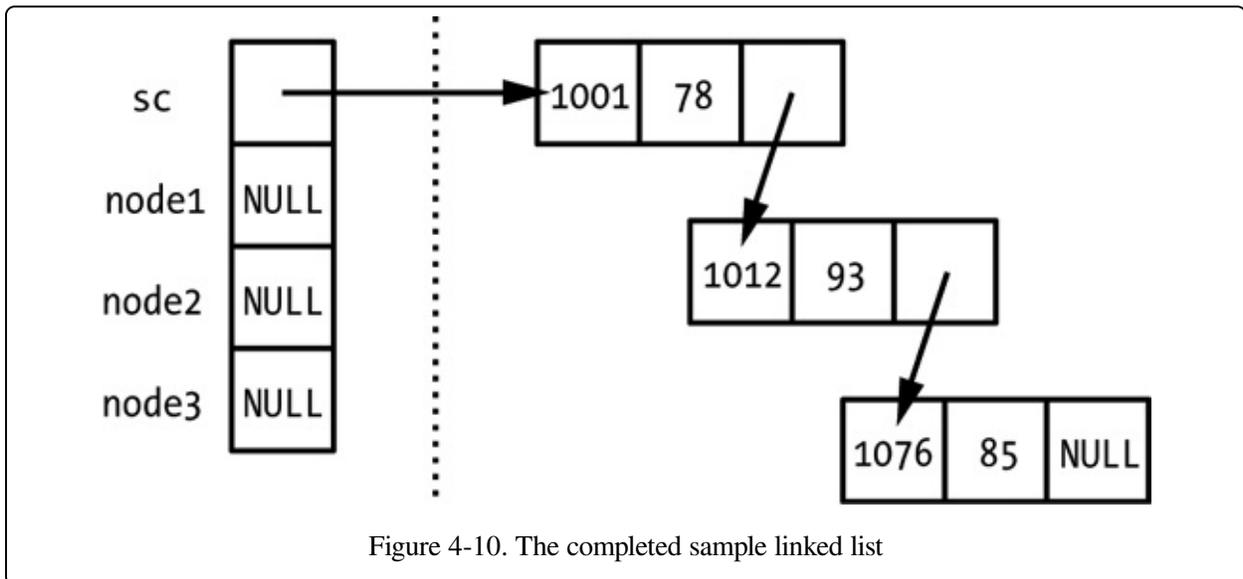
Figure 4-10. The completed sample linked list
